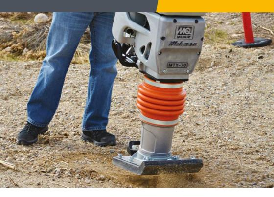
Trench Rammers / Jumping Jacks are ideal for compacting material where space is tight around obstacles.
