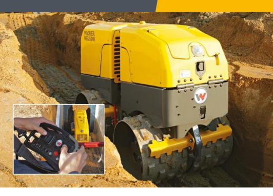
These rollers feature an articulating joint which increases manoeuvrability while a low centre of gravity improves stability. Safety features include operator alert of any close persons/objects. The sheepfoot drum design acts also to provide traction.
