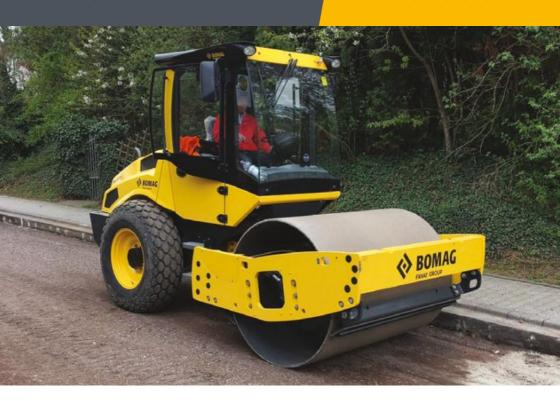
Our range of Compact Construction Rollers feature front mounted Vibrating Drums and rear drive tyres.
