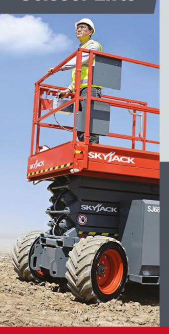
Rough Terrain Scissor Lifts are ideally suited for outdoor tasks where additional traction and stability is required to operate on uneven terrain. Each Scissor Lift is fitted with outriggers to level the machine. With suitable ventilation, Rough Terrain Scissor Lifts can operate inside meaning greater lift capacity and stabilisation over typical Electric Scissor Lifts.
