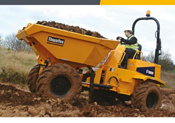
Large Articulated Wheeled Dumpers are ideal for soft and rough terrain. All Dumper units feature swivel skips allowing maximium efficiency on site.
